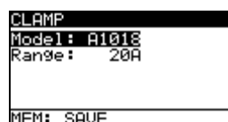
Figure 4.13: Configuration of current clamp measuring input
