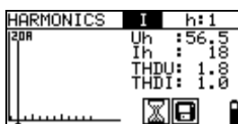
Figure 5.49: Examples of Harmonics measurement results
