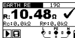
Figure 5.38: Example of earth resistance measurement result
