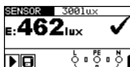
Figure 5.65: Example of illumination measurement result
