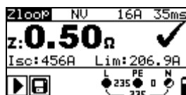
Figure 5.28: Example of loop impedance measurement result
