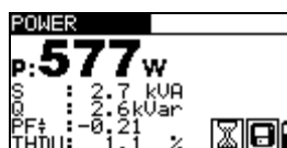
Figure 5.47: Power measurement results
